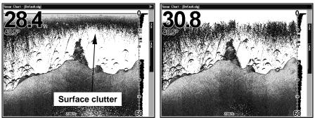
In the illustration on the left, Surface Clarity is turned off. The view on the right shows Surface Clarity set on high.
